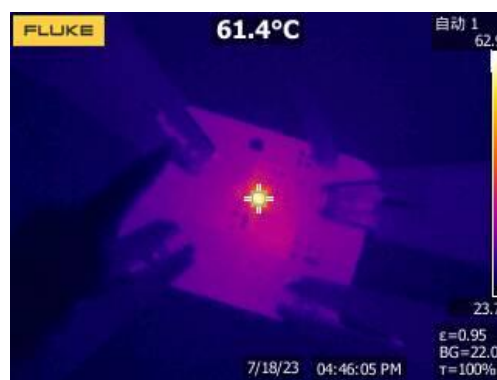
Figure 20. Thermal, V_{IN}=5V , V_{OUT}=1.2V , I_{LOAD}=3A
